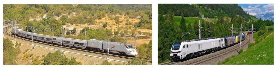
Diesel\* trailers allow electric passenger and freight trains to use non-electrified tracks \* Battery or Hydrogen Fuel Cells in future
