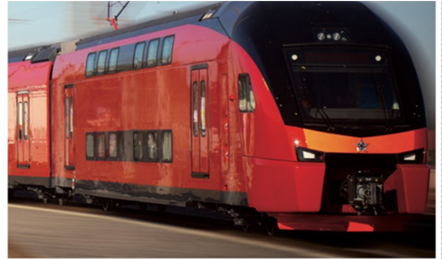
Stadler KISS regional commuter trains have high comfort, top speeds of 160 km/hr and can seat from 250 to 1000 passengers
