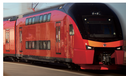
Stadler KISS regional commuter trains have high comfort, top speeds of 160 km/hr and can seat from 250 to 1000 passengers
