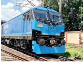
These locomotives are state-of-the-art insulated gate bipolar transistors (IGBT) based three-phase drive.
