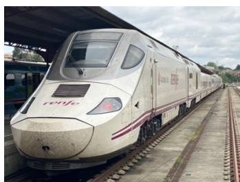
Talgo 250 Dual changes gauge, tilts, and can operate on non-electrified track
