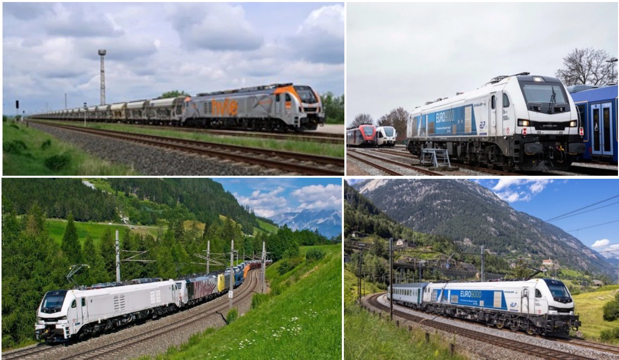
Euro Dual and Euro 9000 bi-mode locomotives handle both fast freight and passenger services in electrified or non-electrified territory.
