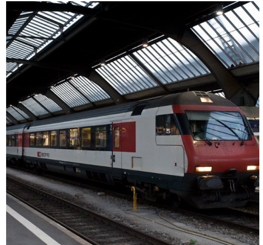
Typical Swiss Intercity Train, showing Driving compartment in rear coach, allowing fast turnaround at terminals.
