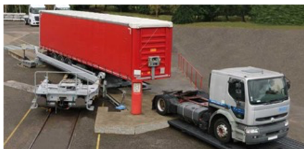
“Modalohr” system for “Rolling Highway” intermodal operation
