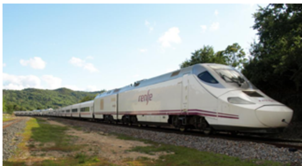
Talgo’s 250 Dual has tilting and gauge-changing ability, and operates at up to 250 km/hr on electrified, and 180 km/hr on non-electrified lines [x/v]
