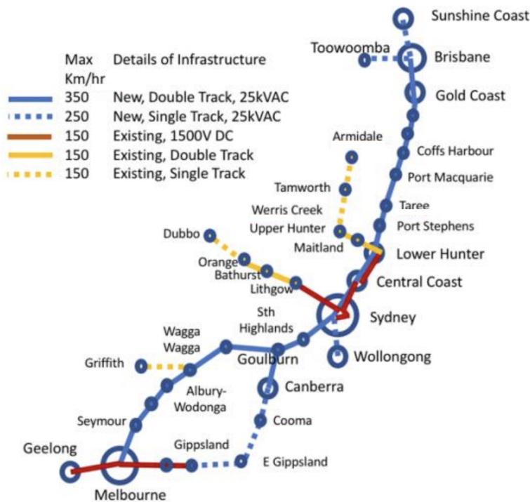
Figure 33: Potential long-term network infrastructure
