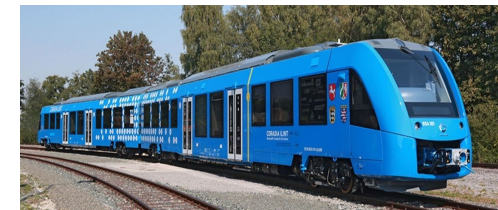
Alstom Coradia iLint hydrogen powered commuter train carries 150 seated passengers up to 1,000km at up to 140km/h
