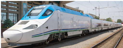
Talgo 250 Dual has both diesel and electric power, tilting capability and a top speed of 250km/h
