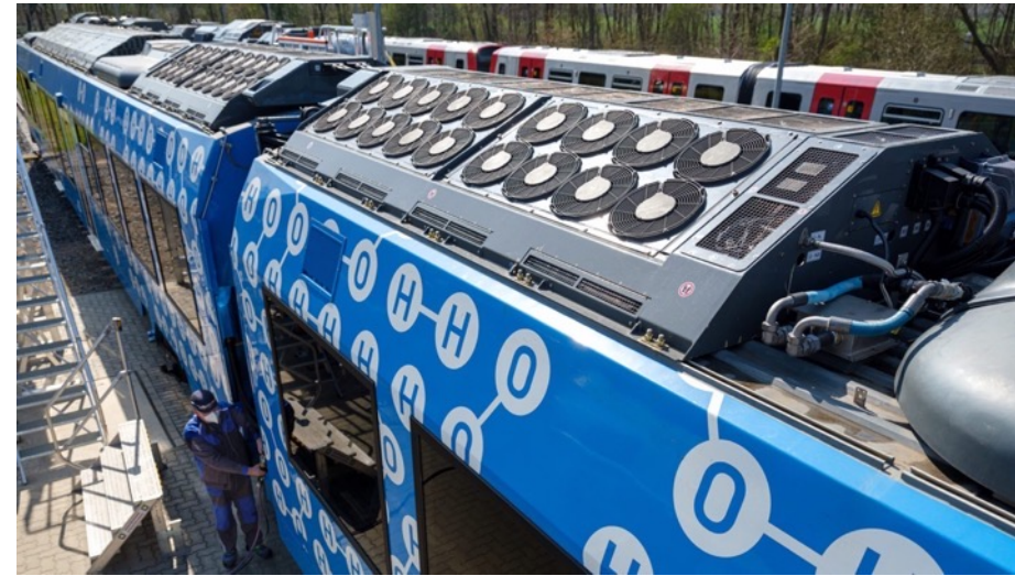
Hydrogen-powered fuel cells on the roof of an Alstom Coradia I-Lint train, already in service in Germany and elsewhere in Europe.
