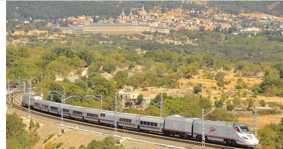
Above: Talgo 250 Dual has both diesel and electric power, has tilting capability and a top speed of 250 kph. . Talgo are working on a hydrogen / electric dual powered train.
